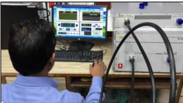
PIM(Passive Intermodulation) TESTING
